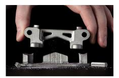
Ceramic Release Layer with Anti-Mold Lock
