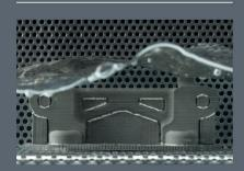
The green part is immersed in proprietary debind fluid, dissolving primary binder and creating an open-pore channel structure throughout the part in preparation for sintering.
