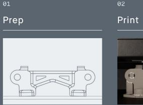
Secure, web-based software constructs build plans from STL or CAD files, automatically generating supports and control parameters based on part geometry and material.
