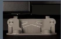
Layer by layer, a green part is shaped by extruding bound metal rods—metal powder held together by wax and polymer binders—in a process called Bound Metal Deposition™.
