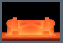
As the part is heated to temperatures near melting, remaining binder is removed and metal particles fuse together causing the part to densify up to 96-99.8%.
